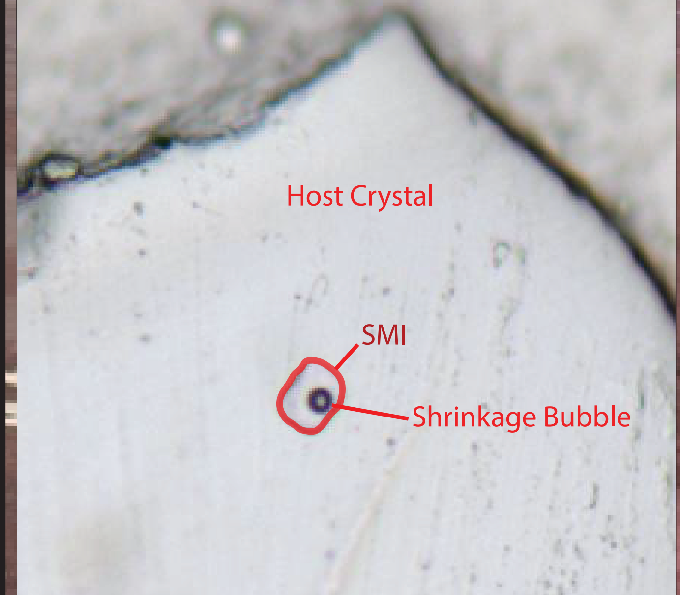
Silicate Melt Inclusions (SMI) are little volumes of magma trapped during crystal growth in a magma chamber and record pre-eruptive chemical compositions, including volatiles. When initially formed, SMIs act as a closed system, recording the composition of the melt at the time of entrapment.
