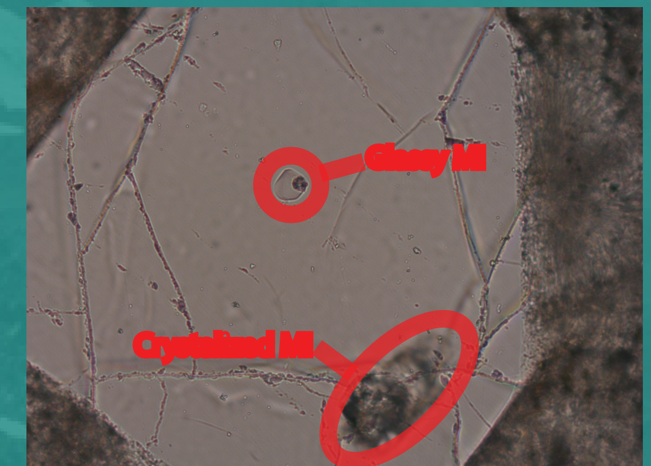
Melt inclusions (MI) hosted in euhedral quartz. Glassy inclusions appear completely clear or include a shrinkage bubble that contains a vapor phase. These inclusions are homogeneous. Crystallized inclusions appear dark and sometimes contain visible microlites and phenocrysts. These inclusions require rehomogenization.
